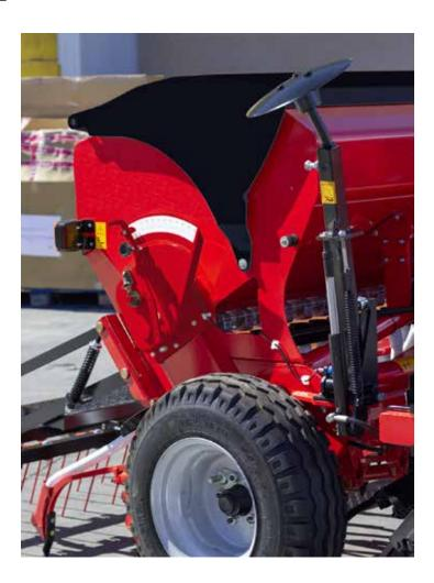
In order to transport the machine, it is essential to fold the track markers so they stay in a vertical position and pin them to the transport bracket using a lynch pin. This will prevent them from lowering during transit.
