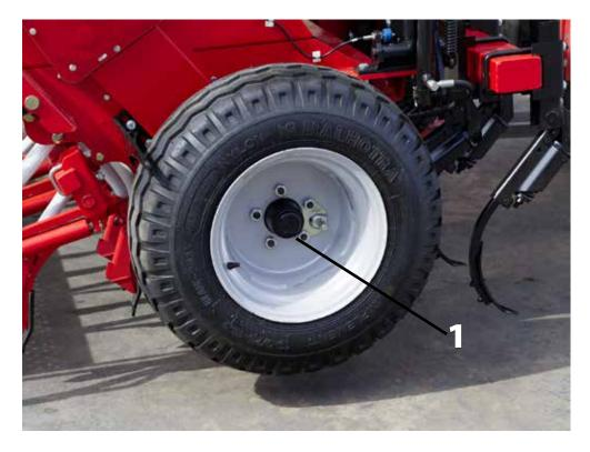
The central adjuster spindle. Use solid calcium grease (2)
