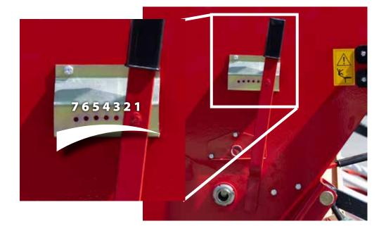
The base flap lever (placed on the left side of the hopper) has 7 positions
