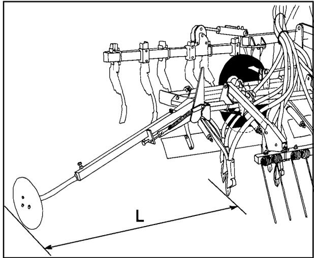
$$L = \frac{\text{ancho labor sembradora} - \text{ancho vía tractor} + 12,5}{2}$$
