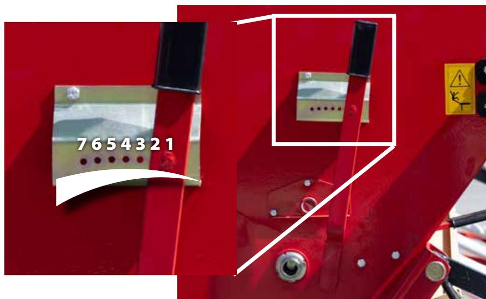
The base flap lever (placed on the left side of the hopper) has 7 positions
