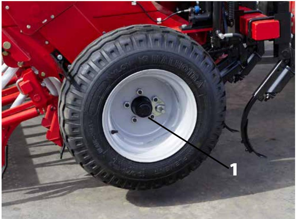
*The central adjuster spindle. Use solid calcium grease (2)*
